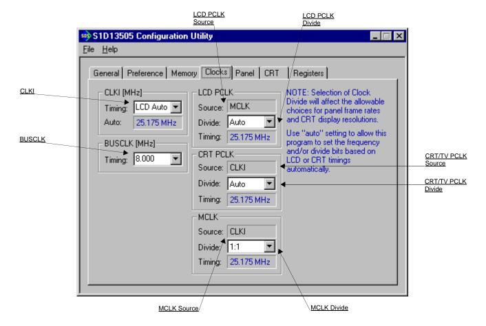
The Clocks tab is intended to simplify the selection of input clock frequencies and the source of internal clocking signals. For further information regarding clocking and clock sources, refer to the *S1D13505 Hardware Functional Specification*, document number X23A-A-001-xx.
