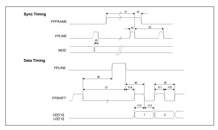
Figure 7-35: 16-Bit Single Color Passive LCD Panel A.C. Timing
