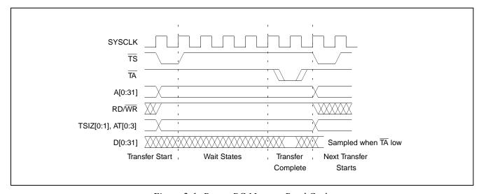
Figure 2-1: Power PC Memory Read Cycle
