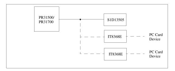
Figure 5-1: IT8368E Implementation Block Diagram
