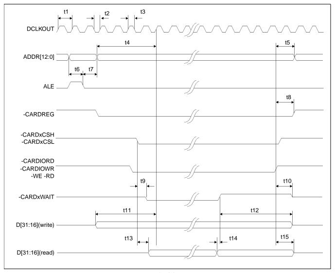
Figure 7-8: Philips Timing
