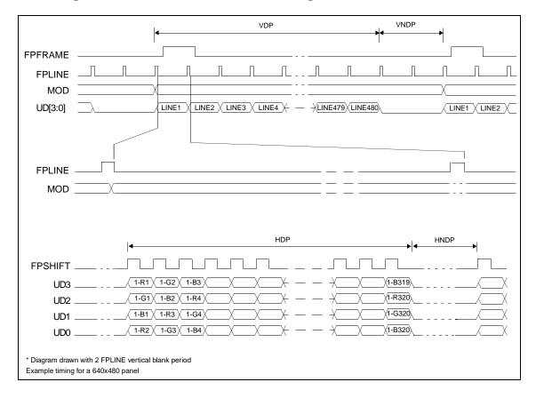
Figure 7-28: 4-Bit Single Color Passive LCD Panel Timing
