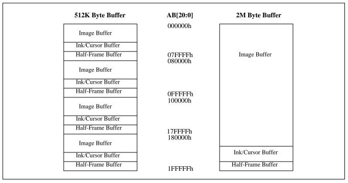
Figure 9-1: Display Buffer Addressing
