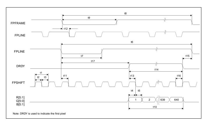
Figure 7-43: TFT/D-TFD A.C. Timing
