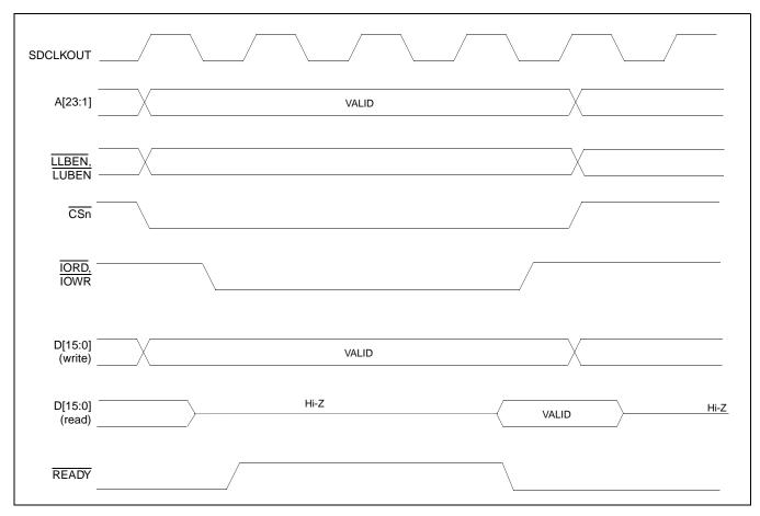
Figure 2-1: NEC V832 Read/Write Cycles
