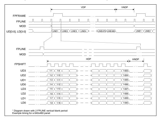
Figure 7-26: 8-Bit Single Monochrome Passive LCD Panel Timing
