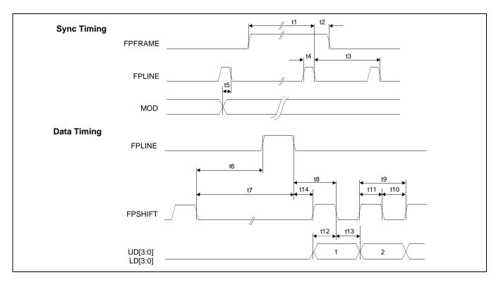
Figure 7-39: 8-Bit Dual Color Passive LCD Panel A.C. Timing
