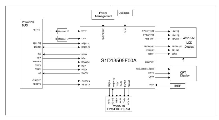
Figure 3-9: Typical System Diagram (Power PC Bus)
