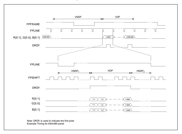
Figure 7-42: 16-Bit TFT/D-TFD Panel Timing
