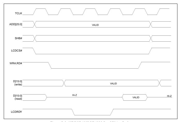
Figure 2-1: NEC VR4102/VR4111 Read/Write Cycles
