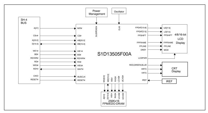
Figure 3-1: Typical System Diagram (SH-4 Bus)
