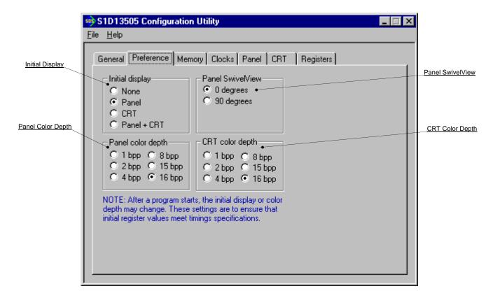
The Preference tab contains settings pertaining to the initial display state. During runtime the display or color depth may be changed.
