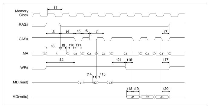
Figure 7-19: FPM-DRAM Read-Write Timing
