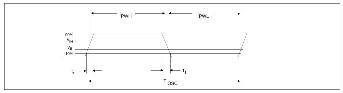
Figure 7-11: Clock Input Requirement
