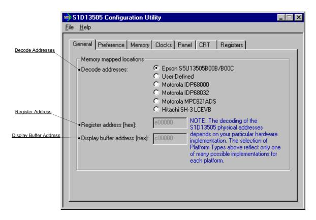
The General tab contains S1D13505 evaluation board specific information. The values presented are used for configuring HAL based executable utilities. The settings on this tab specify where in CPU address space the registers and display buffer are located.
