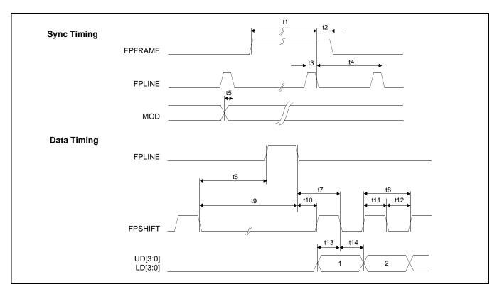
Figure 7-27: 8-Bit Single Monochrome Passive LCD Panel A.C. Timing
