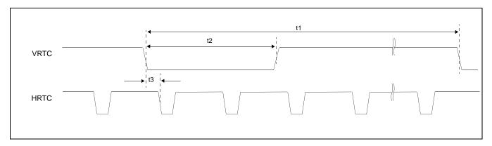
Figure 7-45: CRT A.C. Timing
