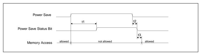
Figure 7-23: Power Save Status and Local Bus Memory Access Relative to Power Save Mode
