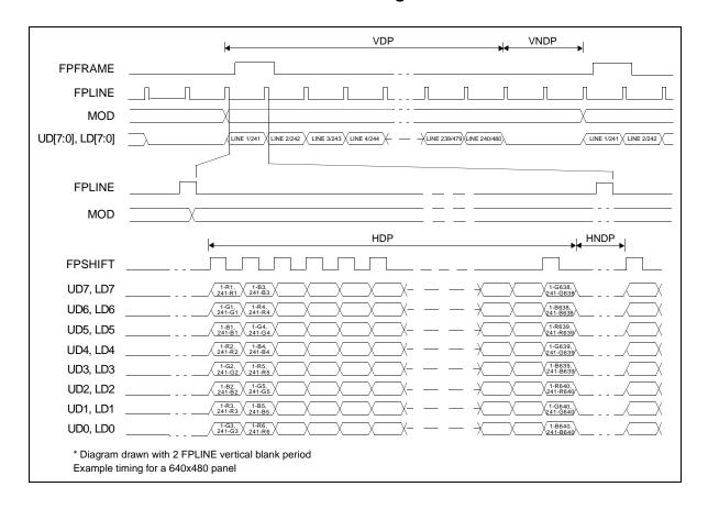
Figure 7-40: 16-Bit Dual Color Passive LCD Panel Timing
