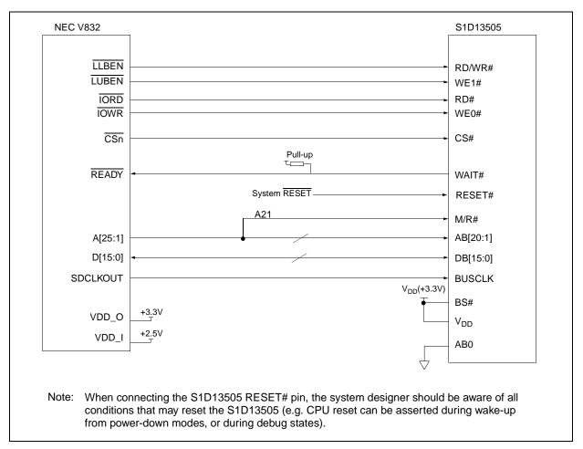
Figure 4-1: NEC V832 to S1D13505 Configuration Schematic
