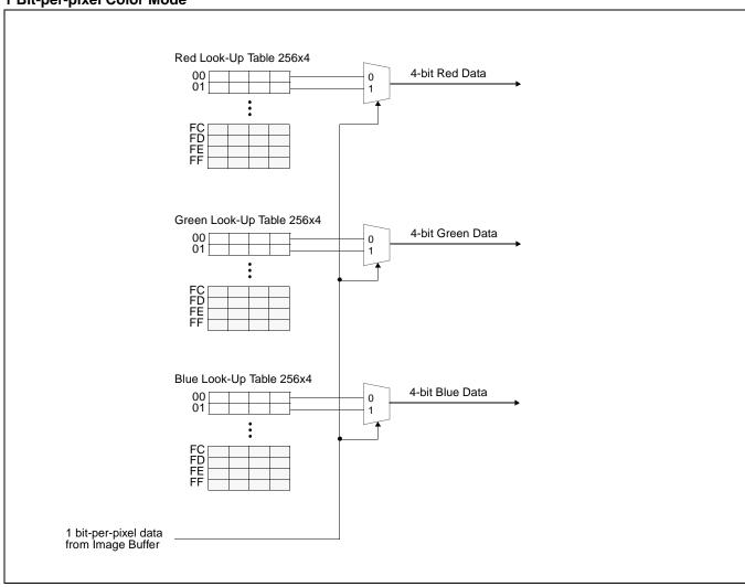
Figure 11-4: 1 Bit-per-pixel Color Mode Data Output Path
