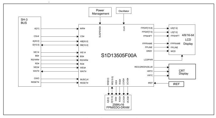
Figure 3-2: Typical System Diagram (SH-3 Bus)
