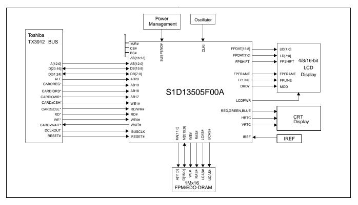
Figure 3-8: Typical System Diagram (Toshiba TX3912 Bus)
