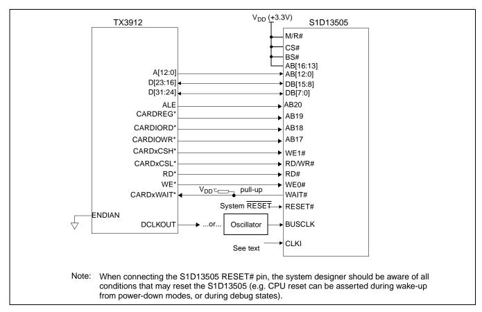
Figure 4-1: Typical Implementation of Direct Connection
