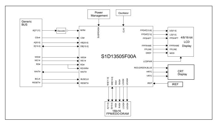
Figure 3-5: Typical System Diagram (Generic Bus)
