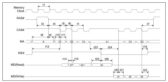
Figure 7-15: EDO-DRAM Read-Write Timing
