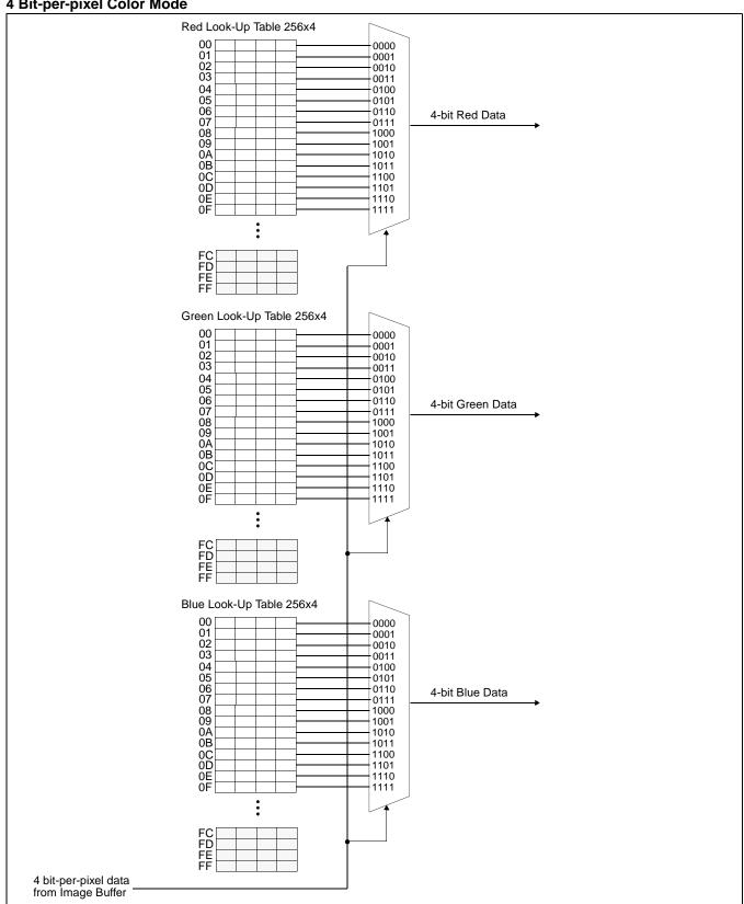
Figure 11-6: 4 Bit-per-pixel Color Mode Data Output Path
