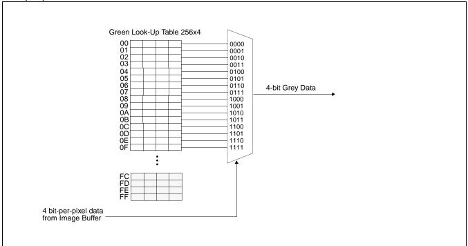
Figure 11-3: 4 Bit-per-pixel Monochrome Mode Data Output Path
