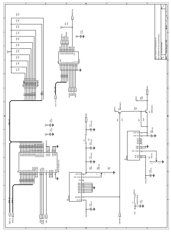
Figure 2: S1D13505B00C Schematic Diagram (2 of 4)
