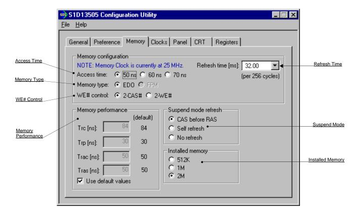
The Memory tab contains settings that control the configuration of the DRAM used for the S1D13505 display buffer.
