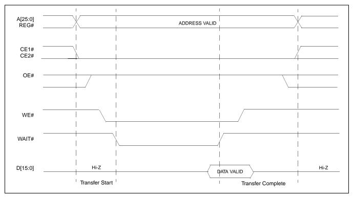
Figure 2-2: illustrates a typical memory access write cycle on the PC Card bus.
