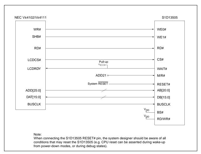
Figure 4-1: NEC VR4102/VR4111 to S1D13505 Configuration Schematic
