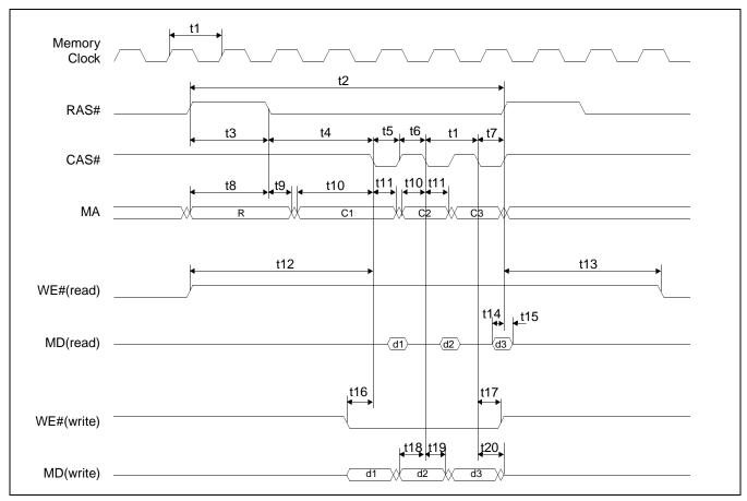
Figure 7-18: FPM-DRAM Read/Write Timing
