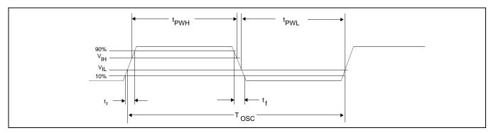
Figure 7-9: Clock Input Requirement
