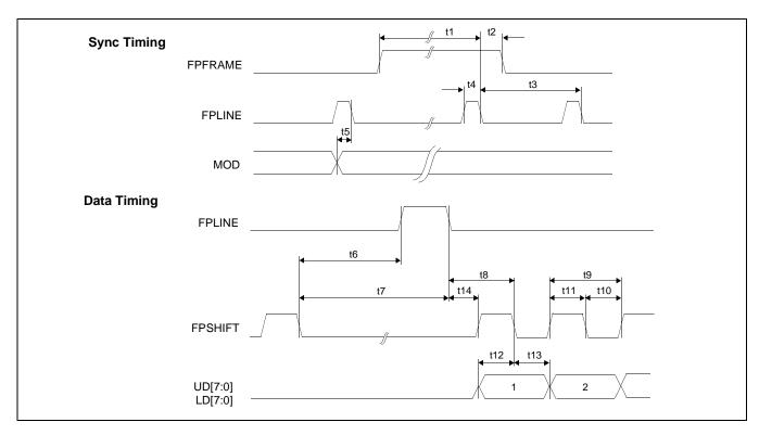
Figure 7-41: 16-Bit Dual Color Passive LCD Panel A.C. Timing
