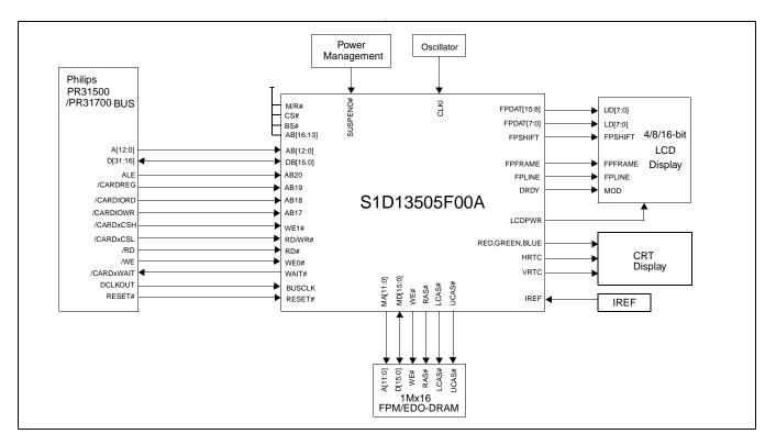
Figure 3-7: Typical System Diagram (Philips PR31500/PR31700 Bus)
