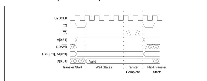
Figure 2-2: "Power PC Memory Write Cycle" on page 10 illustrates a typical memory write cycle on the Power PC system bus.
