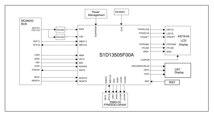
Figure 3-3: Typical System Diagram (MC68K Bus 1, 16-Bit 68000)
