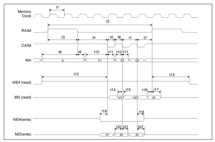
Figure 7-14: EDO-DRAM Read/Write Timing
