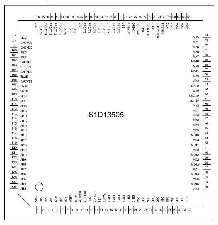
Figure 5-1: Pinout Diagram
