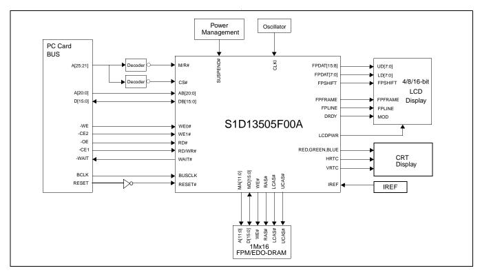
Figure 3-10: Typical System Diagram (PC Card (PCMCIA) Bus)
