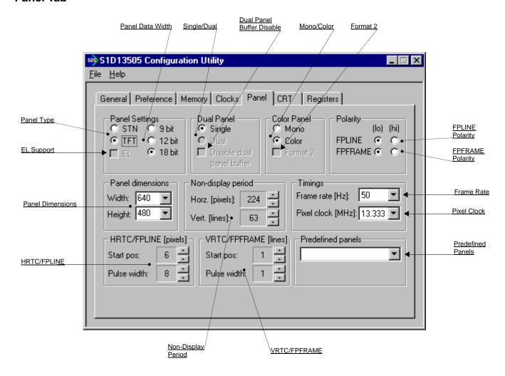
The S1D13505 supports many panel types. This tab allows configuration of most panel settings such as panel dimensions, type and timings.
