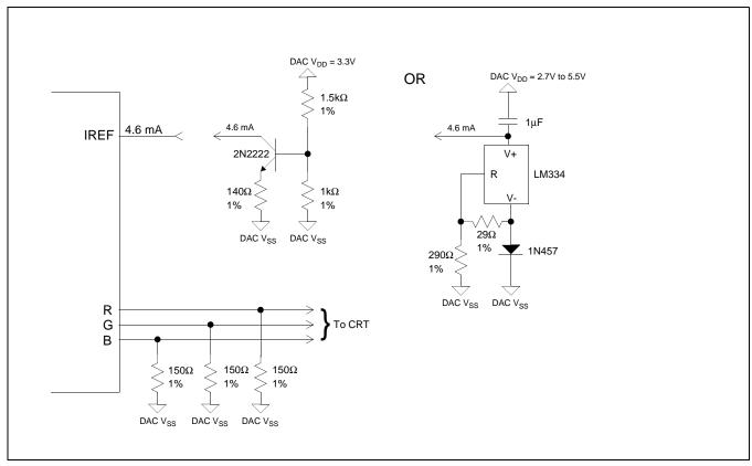
Figure 5-3: External Circuitry for CRT Interface
