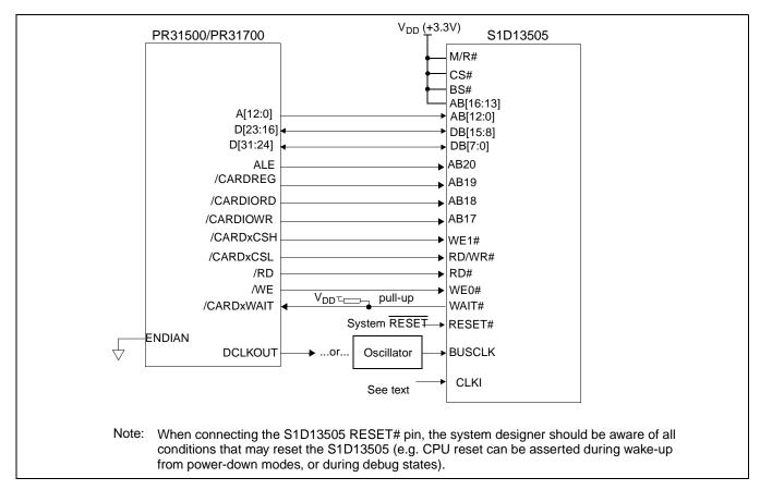
Figure 4-1: Typical Implementation of Direct Connection
