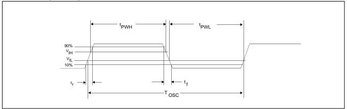
Figure 7-13: Clock Input Requirement
