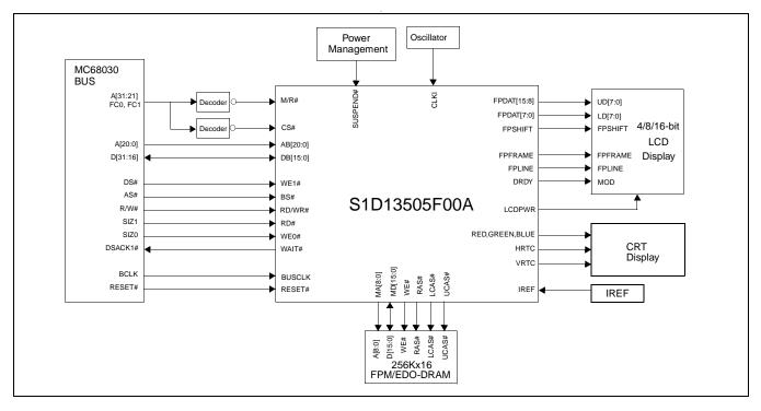
Figure 3-4: Typical System Diagram (MC68K Bus 2, 32-Bit 68030)
