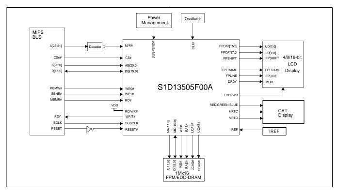
Figure 3-6: Typical System Diagram (NEC VR41xx (MIPS) Bus)
