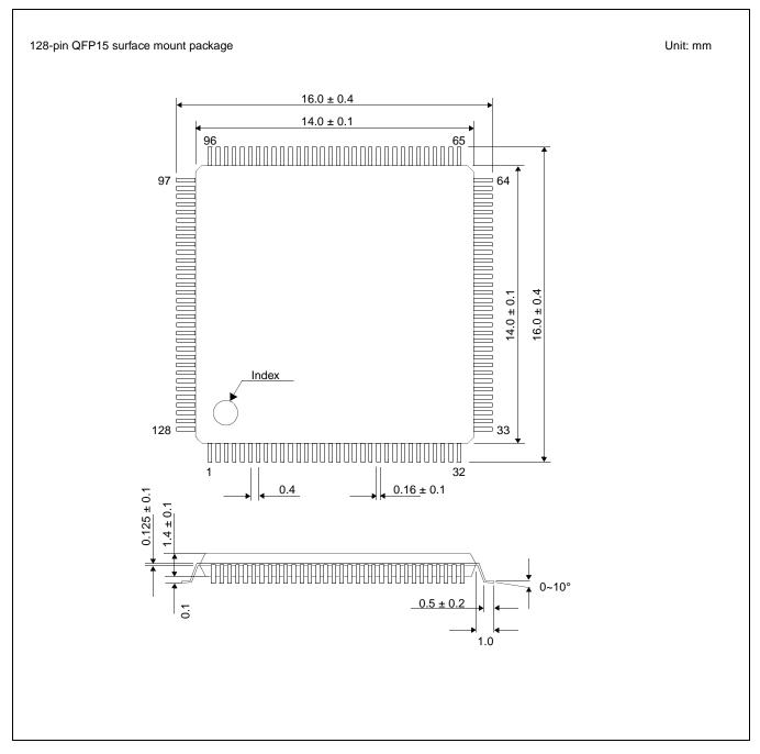
Figure 16-1: Mechanical Drawing QFP15
