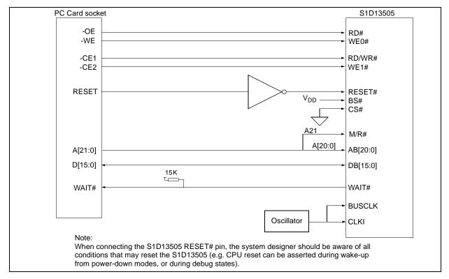
Figure 4-1: Typical Implementation of PC Card to S1D13505 Interface
