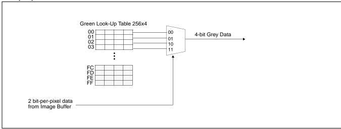
Figure 11-2: 2 Bit-per-pixel Monochrome Mode Data Output Path
